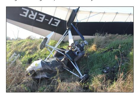
**Photo No. 1**: Final resting position of aircraft. Note ladder bottom left.
